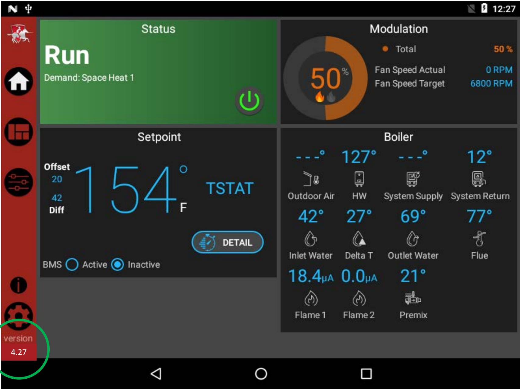
At this point, you will be asked if you would like to apply the update found on the USB drive. Confirm the update to install on the boiler. Once uploaded, the display will turn off and reboot. When the screen powers back on and loads, the update is complete.
